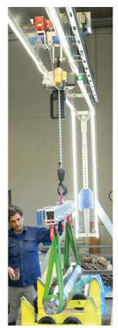
No personal effort is required when working with the aluminium gantry crane with electrically movable trolley.
