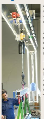
easier and requires less physical effort from the user. No personal effort is required when working with the aluminium gantry crane with electrically movable trolley.
